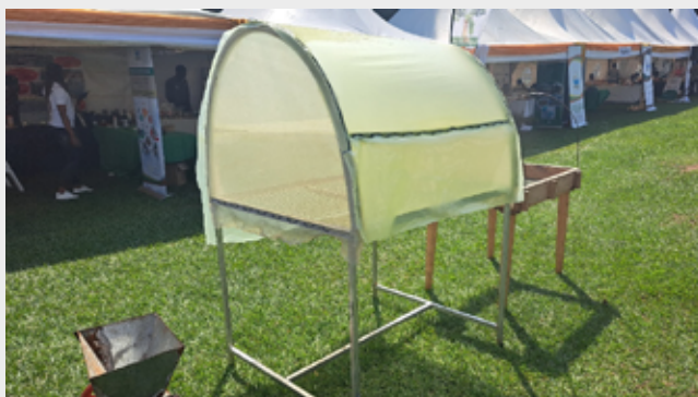
Fig 5 The hybrid solar drying technology for Post-harvest management
